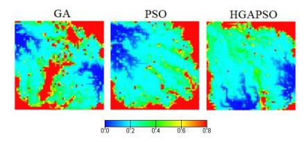
Fig. 12. Oil saturation maps for best optimization runs of GA, PSO and HGAPSO algorithms (case 3).
