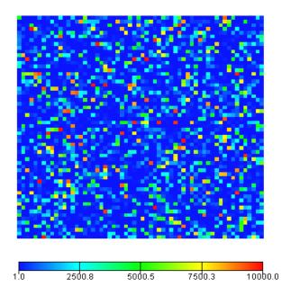
$\textbf{Fig. 9.} \ \ \text{Permeability distribution for reservoir model of synthetic case 3}.$
