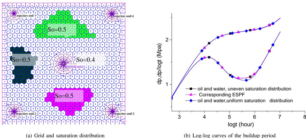
Fig. 6. Log-log curves of the buildup period.
